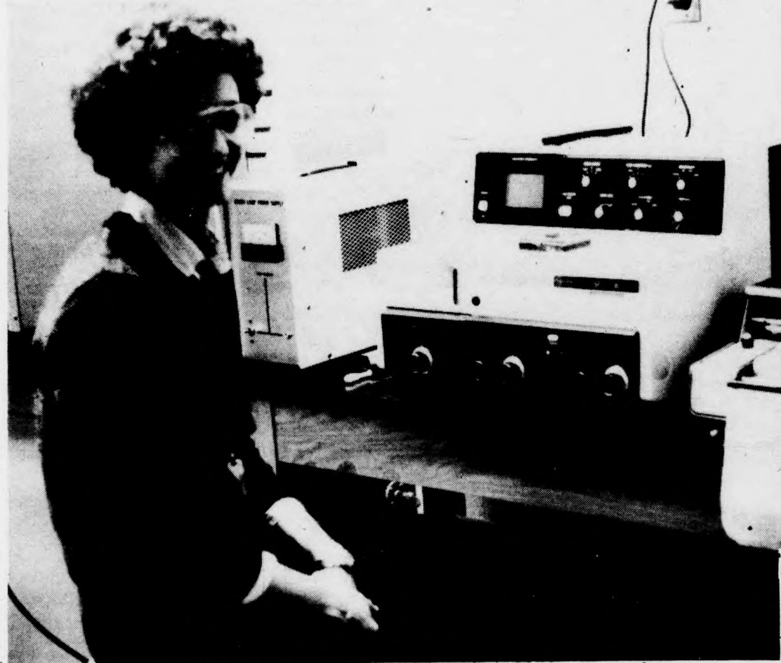
Silvia Licoccia using a spectrofluorometer to measure the lifetime of a possible catalyst
