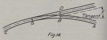
While the writer realizes that it is better practice to place the frog end of the connecting curve at the heel of the frog, to impose that condition in the above problem would complicate it beyond measure. In inserting 10 or 15-ft. frogs in a curved track, the trackmen cannot help slightly changing the original alinement of the track at that point, and energy spent in making a closer solution than that outlined above will surely be wasted.
