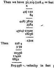
819.956 - velocity in feet per second, which steam at 60 lbs. will flow into the atmosphere at constant density.
