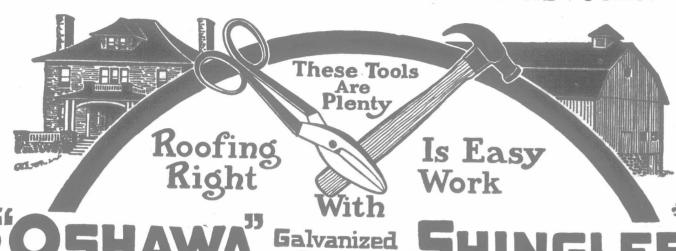
Put them on with no tools but a hammer and tinner's shears,—can't go wrong. They lock on all four sides, are self-draining and watershedding on any roof with three or more inches pitch to the foot. Make buildings fire-proof, weatherproof and proof against lightning. Cost
