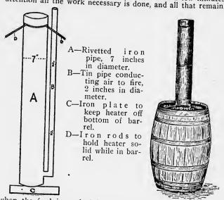
when the feed is cooked is to remove the heater and the grain will have swelled up enough to take its place, leaving a barrel full of feed. The heater proper cost Mr. Reilley but \$1.50, and was made in town for that price.
