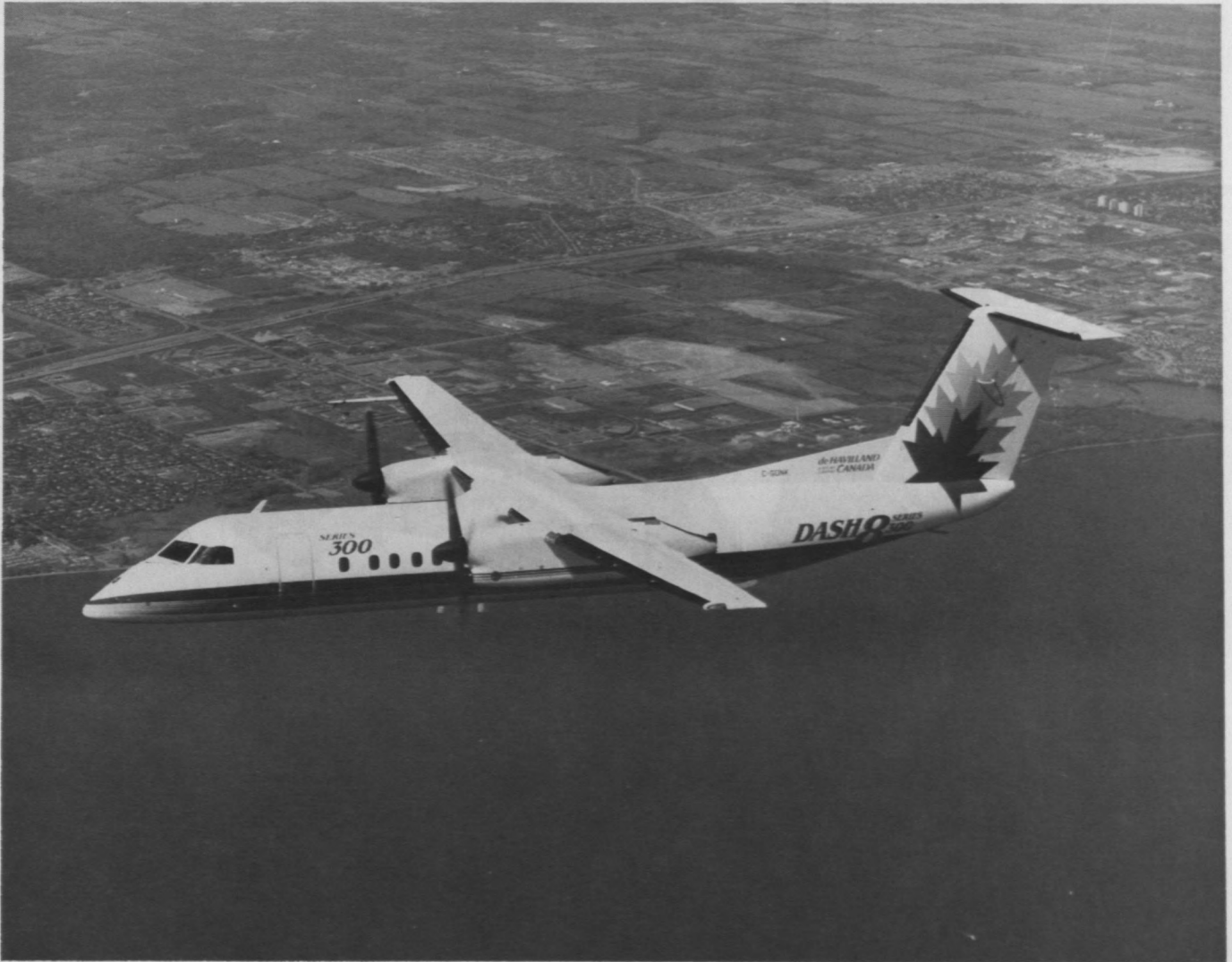
Figure 5. The Boeing Dash 8 Series 300 provides a large volume platform, with room for 16 passengers or more as well as a full complement of sensors. The aircraft could be used to transport on-site inspection teams as well as being a sensor platform. (Courtesy of Boeing Canada, de Havilland Division)
