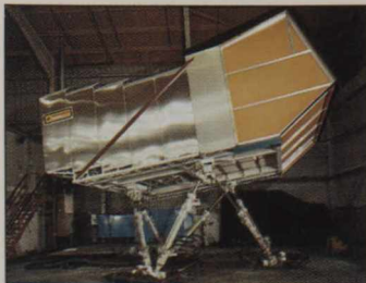
Exterior of the simulator showing the hydraulic legs used to give the theatre its simulated motion.
