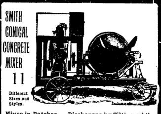
Mixes in Batches. Discharges by Tilting while Running. Mounted on Skids or Trucks. Catalogue on Application.
