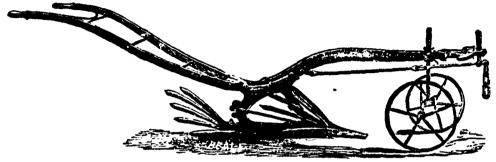
With a pair of horses, three to four acres of potatoes can be raised in a day; it leaves fewer in the ground than when dug by hand, and raises the roots without bruising or scratching the skins. For earthing up potatoes, it will be found a better implement than the ordinary ridging plough, as it throws the earth lightly on to the plants, and the draught is easier. It may readily be converted into a ridging plough by adding a pair of breasts.
