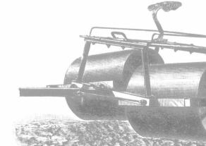
It rolls all the ground, no matter now There is no axle shaft, no strair consequently no wear. It is eas olled between the drums. no strain,
