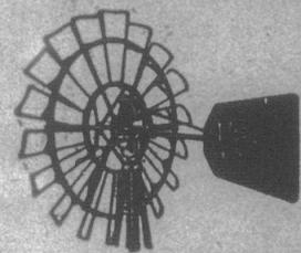
when fitted with GRAPHITE bearings. They run without oil; no more CLIMBING TOWERS TO OIL BEARINGS.
