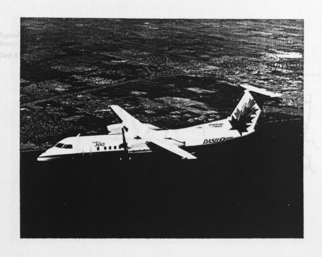
Figure 21. The de Havilland Dash 8 Series 300 provides a platform with room for 16 passengers or more as well as a full complement of sensors. Based from a central location in Europe, the Dash 8 could reach any target within the "Atlantic to the Urals" region within six hours without refueling. The Dash 8's airfield performance would permit operations from most airfields in Europe. (Courtesy of Boeing Canada, de Havilland Division)
