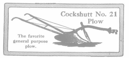
You often need a plow which can turn to almost any kind of work. In other words, a general-purpose plow. The "Cockshutt" No. 21 is probably the best known and most used of any Canadian - made walking plow. It is easily held and controlled by the long handles. The mold board is so shaped that stones do not harm or throw it out. It cuts evenly and well from 10-12 inches wide and from 4-8 inches deep.
