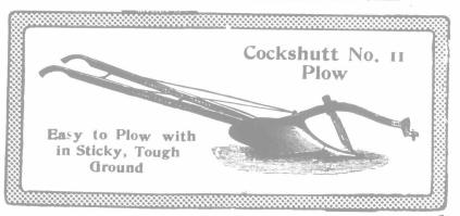
The No. 11 Plow is built specially for clay land. It has been on the market the past three seasons, and wherever it has been introduced has given thorough satisfaction. It will cut a clean furrow 5 to 8 inches deep and 6 to 9 inches wide, and on account of fairly lengthy handles is easily controlled. This plow is strongly built, and the steel board will clean nicely. It is fitted when shipped with chilled share, extra share being also supplied.
