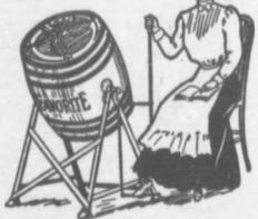
The "Favorite" can be operated by hand or foot, or both—while you are sitting in a chair. Easier than a sewing machine. Steel roller bearings and other improvements make it the ideal churn for farms and dairy. 8 sizes, to churn from ¼ to 30 gallons of cream.
