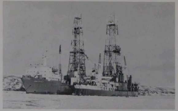
The Deepsea Miner II (left), a converted ore carrier, is used for tests on deep-ocean mining of manganese, nickel, copper and cobalt nodules. The Canmar Explorer III is a Dome Petroleum oil exploration rig.
