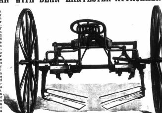
Knives can be Locked in any Desired Position.
