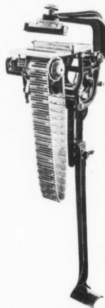
Addressograph with Endless Chain of Addresses Suspended on the Revolving Drum.
