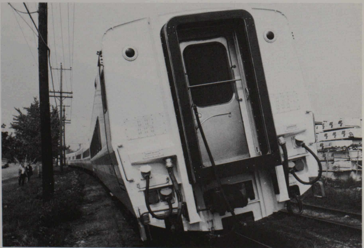
The unique banking system of Bombardier's LRC trains allows them to negotiate sharp curves at high speed.
