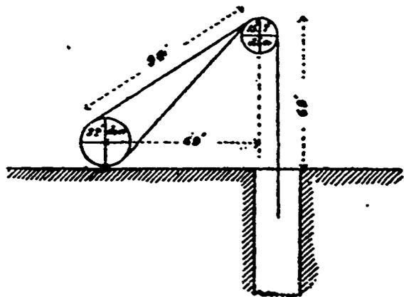
barrel of the drum, the angle from the pulley-line will be about 1° 7' on each side. It was feared that the round ropes would not coil properly on the drum, but to avoid that they grooved the lagging, and it is satisfactory to know that it is successful, and further that it has reduced the side friction at the drum to the lowest possible degree. They wind from a depth of 530 yards, the speed being about 45 seconds, or about 24 miles an hour.
