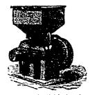
These mills grind all kinds of grain, as well as phosphates, quartz, plaster, clay, dc., dc.
