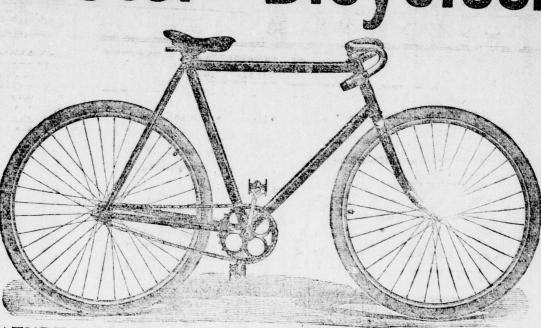
WINCHESTER FEATURES-Flush joints, steel forged connections, tool steel bearings, handle and saddle post binders, Dunlop tires, 3-ply rims—an improvement ir every line.
