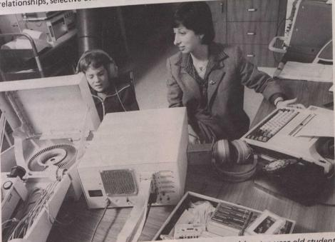
Dr. Elaine Pressman begins auditory discrimination testing with a ten-year-old student. The system incorporates a random access slide projector, a random access audio unit and a touch-sensitive screen device. The terminal is packaged in portable units which can be easily relocated and reassembled.
