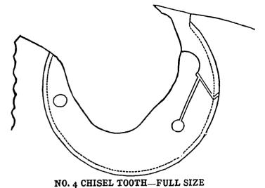
Suitable for Soft, Pitchy Timber, where more throat room is required. A good all round tooth. Saws made with this tooth from 5 to 9 gauge.
