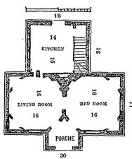
A glance at the plan of the first floor will show that its accommodation is very compactly arranged. By placing all the flues in one stack, no heat is lost in winter; and by cutting off the corners of the two principal rooms, convenient closets are afforded. As, in a house of this class, the kitchen is usually the room most constantly occupied by the family, there is no objection
