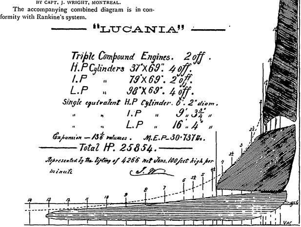
The lengths of the diagrams are in the ratio of the volume swept per stroke of their respective pistons, and the pressures on the original diagrams are plotted to a uniform scale.
