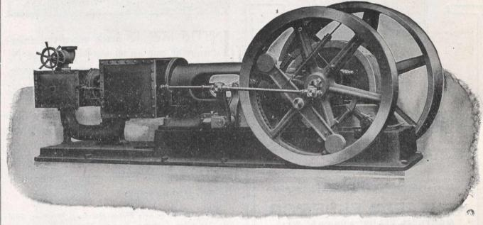
The above cut shows a 19 and 32 by 24 Tandem Compound Automatic McEwen Engine. Four of these are in use in Southern Ontario operating 400 K. W. Generators.
