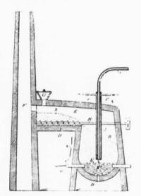
Mr. Ruthenberg makes the important point that during the exposure of the ore to the action of the electric arc a considerable part of any sulphur in the ore is eliminated.
