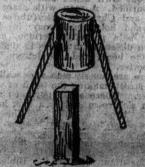
a post hammer, which is the best tool for setting ordinary fence posts I ever saw. Have used one for several years. I made mine from pine wood, but that timber is too light. Can drive an ordinary post into any kind of soil. Two men are to use tool, one man to each handle. Raise up stool and let fall on top of post, one man to stand on one side of post, and the other to stand on opposite side. I got the idea for making this tool from the ordinary pile driver.—J. E. Rotan, in Practical Farmer.
