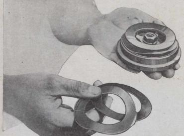
Compressors Light thin steel discs, held to their seats by flat springs of the same material, form the valves of Sullivan WG-6 single stage belted Compres-
