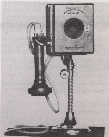
Blake magneto desk telephone, circa, 1880, contained the transmitter invented in 1878 by Francis Blake, which relayed the voice with an improved clarity over any telephone used before this. The Blake was used in Canada until about 1900.
