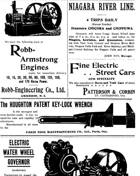
Variations in speed detected by fast running, sensitive Governor Balls. Gate movement instantly set in operation by electric current. Quick and powerful action.
