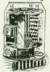
A heating apparatus with from nine to seventeen vertical corrugated cast iron flues or sections forming the fire cylinder and combustion chamber, and having 65 square feet of heating surface to each square foot of grate surface.
