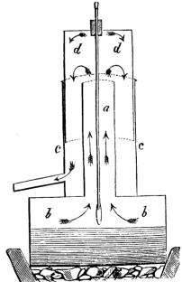
half a gallon, (b) to which is added a tube (a) about three inches in diameter and ten high; exterior to this, but not communication
