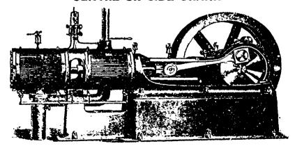
In the Tandem Compound the high pressure cylinder is placed next the frame, and both pistons and cylinder heads may be withdrawn through the low pressure cylinder without disturbing the cylinders, valves or other parts. Both valves are controlled by the governor, so arranged that an equal amount of work is done in each cylinder.
