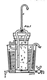
I and I connected together by the double action stop-cock K, with the facest M, the ordinary tub A, the interior surface of which is covered with a serpentine B, B which acts as a cooler, all substantially as and for the purpose set forth.
