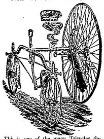
This is one of the many Tricycles the Rudge's turn out. For a single Tricycle it cannot be excelled; the two-track arrangement being much superior to the old three-track affair.
