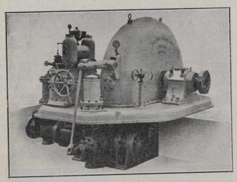
Fig. 3.—Generating Turbines of 6,500 H.P
