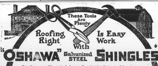
Put them on with no tools but a hammer and tinner's shears, -can't go wrong. They lock on all four sides, are self-draining and watershedding on any roof with three or more inches pitch to the foot. Make buildings fire-proof, weatherproof and proof against lightning. Cost least in the long run. Made of 28gauge toughened sheet steel-only one quality used and that the bestbent cold and double-galvanized. Last longer with no painting than any other metal shingles heavily-
