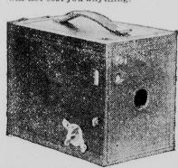
Description—For rectangular pictures 2½ x 3½ inches. Capacity, 6'exposures. Size of camera, 5½ x 4 x 3½ inches. Weight 13 ounces. Lens, Meniscus, fixed 4½-inch focus. Shutter, Eastman rotary, with three stops. Two finders.
