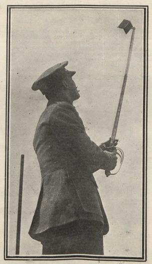
The only time a British soldier turns his back to the enemy is when he is using his pocket peris-cope. This is a simple little instrument consisting of two mirrors at right angles, and arranged so that it can be adjusted to a sword or a bayonet and held above the parapet of a trench without danger to officer or private.
