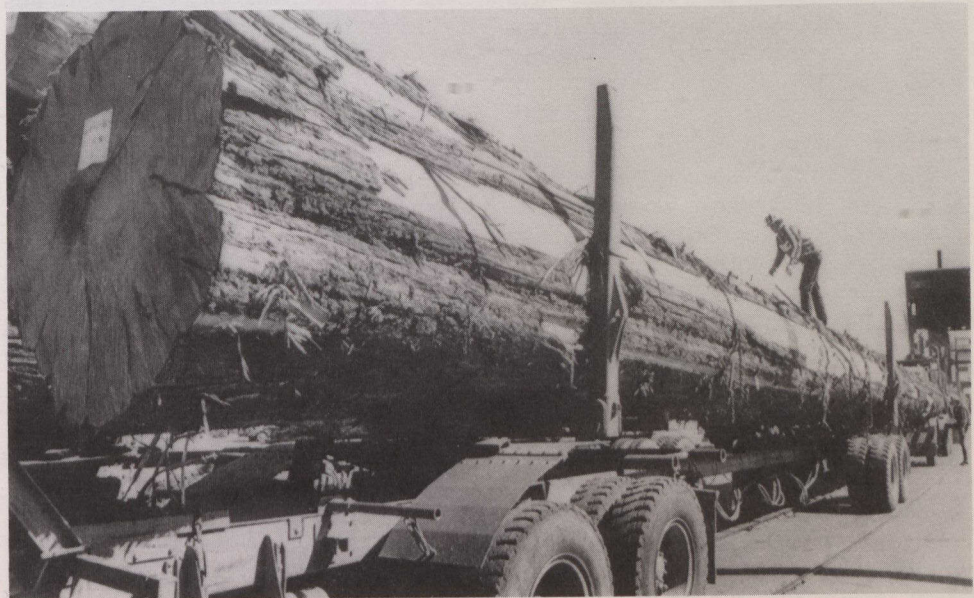
Nineteen giant western red cedar logs arrived recently in Vancouver intended for construction at Expo 86's Folklife Festival. The logs, felled in the Alberni region of Vancouver Island, will be used to form the roof beams, lintels and columns for the Native Theatre, a West Coast Indian longhouse.
