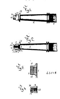
female thread engaging the oppositely-threaded portion of the axle and a male thread engaging the second thread of the washer, substantially as described.
