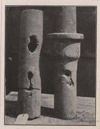
times. The distance is approximately 1,200 feet, that is, the drop of potential from these tracks to the station is one volt per 100 feet. This is altogether excessive, a voltage drop of one-half volt per 300 feet is usually considered large enough. The above condition is responsible for the trouble reported in district No. 4.
