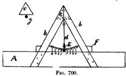
inches from centre board A, and nail other two on the other side of board A; then place the triangle piece, like C, between the four upper ends, indicated by a dotted line; then nail firmly. G indicates an eye fastened under C in centre to tie the line d; F is a piece of board 1 inch thick, 5 inches wide, and long
