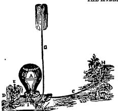
The Hydraulic, or Water Ram, is a very ingenious modern invection; and as economical and useful as it is ingenious. Of course, it is necessary that there should be a running stream within a reasonable distance of the spot where the water is required to be delivered. The principle on which it acts, may be understood from the accompanying cuts and description:-
