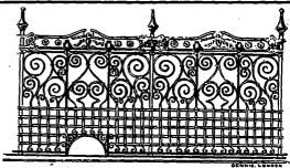
Bank Railings, Tellers' Cages (with roof), Grilles, etc., in iron, steel or brass. DENNIS WIRE AND IRON WORKS LONDON,
