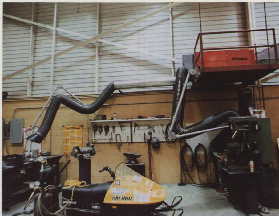
Tykron Industries Ltd. Air standard Model AS4000 for general ventilation or source pick-up.
