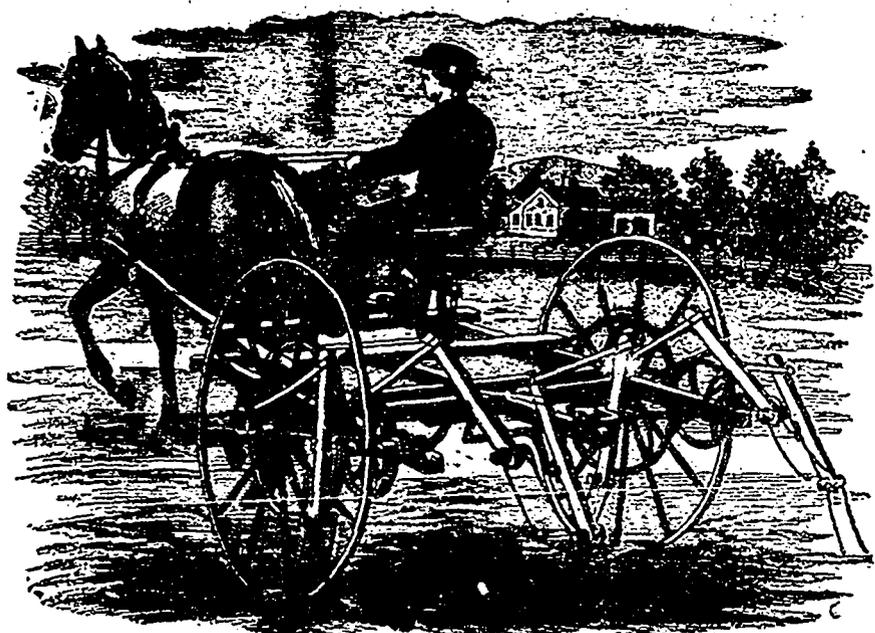
Experience has demonstrated the fact that a good **Hay Tedder** that will thoroughly spread long, heavy grass, taking it up from the bottom, tossing it gently into the air, and leaving it upon the ground in a light, fleecy condition, enables the farmer to take advantage of fair weather, and at least twice the quantity of Hay can be secured, in better condition, than when allowed to remain in the swath.
