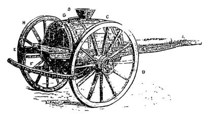
The apparatus for regulating the discharge of liquid manure. Fig. 1.
