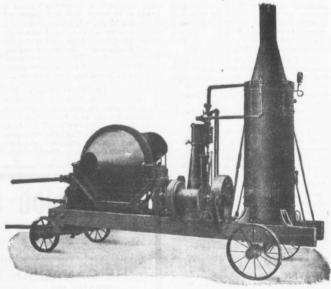
Spirally inclined, they cut away, lift, turn over and pour into a a central tumbling chaos every particle of the material, many times per minute.
